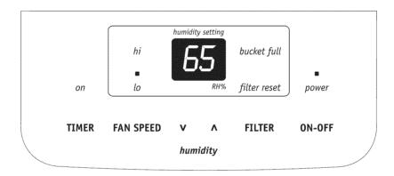
5. The FILTER RESET light will illuminate after 250 hours of operation. At this time refer to the care and cleaning section to remove and clean the filter. Once the filter has been cleaned, to extinguish the light simply press the FILTER button.
