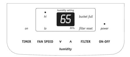
4. You can also use the FAN button to change the fan speed to HIGH or LOW. The indicator light will show the setting you have selected. A higher fan speed will result in quicker moisture removal.
