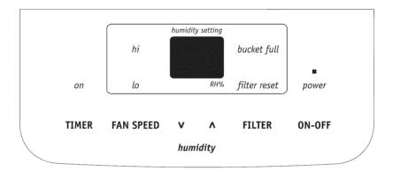
2. To turn the unit on press the ON/OFF button. The unit will run in the factory setting of CONTINUOUS and high fan speed. In the Continuos Mode the unit will only display CO and not the room humidity. It is recommended you leave the unit running in the CONTINUOUS setting for the first three or four days until the sweating and dampness odors have stopped.
