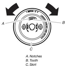
4. Tighten the locking screws and replace knob.
