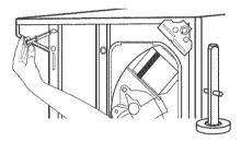
Check adjustability of rear legs by pushing in one leg. The other leg should come out. Check both legs. If they do not move freely, repeat Step 1.
