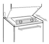
2. If the washer/dryer is not level, prop up the front with a wood block and adjust the feet up or down as necessary. Remove wood block and lower washer/dryer. Repeat this step until the washer/dryer is level.
