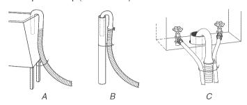
If the water faucets and the drain standpipe are recessed, put the hooked end of the drain hose in the standpipe. Tightly wrap the plastic strap around the water inlet hoses and the drain hose (C above).
