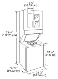
\*Most installations require a minimum 5½" (14 cm) clearance behind the dryer for the exhaust vent with elbow. See "Venting Requirements."
