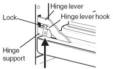
Lock engaged for door removal Figure 1
