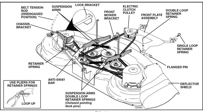
Position front plate assembly between front mower brackets. Raise deck and plate assembly to align holes and insert flanged pins. Secure pins with double loop retainer springs between the plate assembly and mower brackets.
