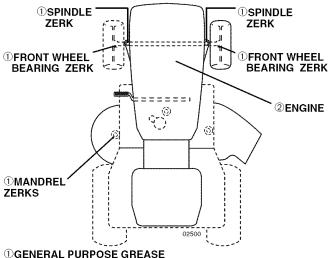
©GENERAL PURPOSE GREASE ©REFER TO MAINTENANCE "ENGINE" SECTION
