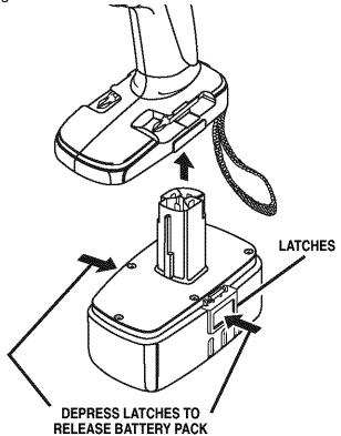
Make sure the latches on each side of the battery pack snap into place and the battery pack is secured in the drill before beginning operation.
