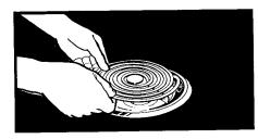
3. Push the surface element terminal into the receptacle. When the terminal is pushed into the receptacle as far as it will go, the surface element will fit into the drip bowl.
