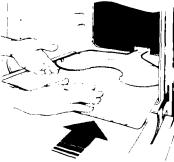
Slide the foil under the bake element.
