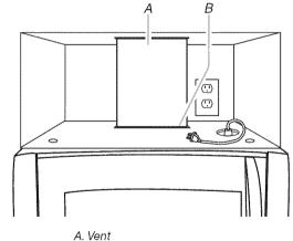
B. Damper assembly (under vent)
