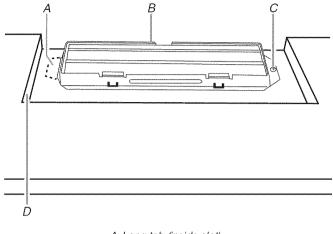
A. Long tab (inside slot) B. Damper assembly C. Mounting screw
