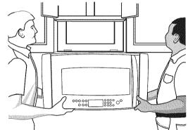
**3.** Using 2 or more people, lift oven and hang it on support tabs at the bottom of mounting plate.
