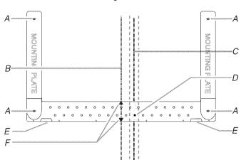
**NOTE:** If wall stud is within 6" (15.2 cm) of the vertical centerline (see "Mark Rear Wall" section), only ventless (recirculating) or roof venting installation can be done.
