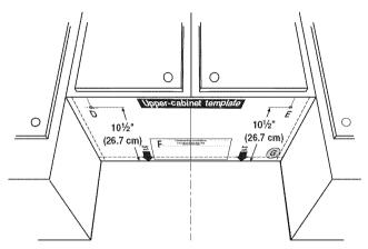
Cut the 1½" (3.8 cm) diameter hole at the circular shaded area "G" on the template. This hole is for the power supply cord.
