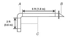
A. One 3 1/4" x 10" (8.3 x 25.4 cm) 90° elbow = 25 ft (7.6 m) B. 1 wall cap = 40 ft (12.2 m)C. 2 ft (0.6 m) + 6 ft (1.8 m) straight = 8 ft (2.4 m)
