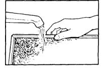
Soak grease filters in hot water and a mild detergent. Scrub and swish to remove embedded dirt and grease. Rinse well and shake to dry.
