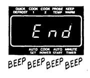
When the cooking time ends, "End" will show on the Display and 4 beeps will sound. (You can stop the beeping by opening the door or by touching CANCEL.) "End" will remain on the Display and a reminder tone will sound every 60 seconds (to remind you that food is left in the oven) until the door is opened or CANCEL is touched. The Display will then show the time of day.
