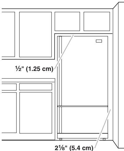
To ensure proper ventilation for your refrigerator, allow for a  $\frac{1}{2}$ " (1.25 cm) space at the top and behind the refrigerator. When installing your refrigerator next to a fixed wall, leave  $2\frac{1}{8}$ " (5.4 cm) minimum on each side (depending on your model) to allow for the door to swing open. If your refrigerator has an ice maker, allow extra space at the back for the water line connections.
