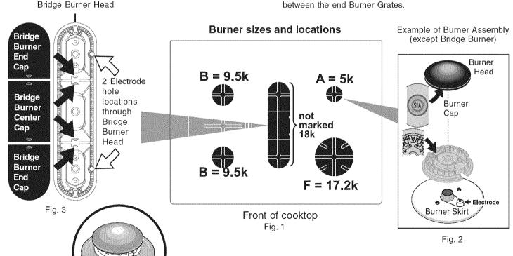
Electrode must align into slot or hole for Simmer Burner Head
