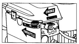
**Step 6** Slide the throttle control to the fast position. Move the choke lever to the "CHOKE" position (only if engine is cool). After starting, move the choke to "RUN".
