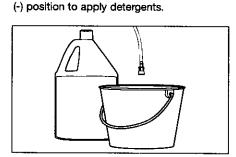
**Step 2** Fill a container with Karcher detergent. Place the filter end of detergent suction tube into the container.
