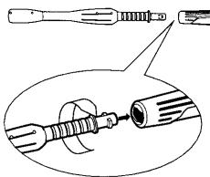
**Step 1** Install the Vario spray wand and set the Vario spray wand to the low pressure setting (-) by turning the wand collar. The wand must be set in the low pressure
