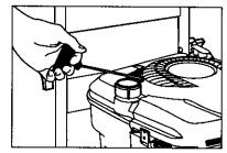
**Step 7** Pull the starter handle. If the engine fails to start after 3 pulls squeeze the trigger gun to release pressure, and repeat step 7.
