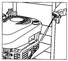
**Step 2** Check oil level. Oil level should always be between the "FULL" and "ADD" marks on the dipstick. Be sure the machine is level when checking the oil level. (Refer to the engine's operating manual for seasonal grades.)
