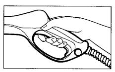
**Step 3** With the engine running, pull trigger to operate unit: Liquid detergent is drawn into the unit and mixed with water. Apply detergent to work area. Do not allow detergent to dry on surface.
