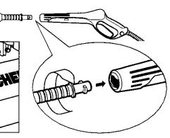
**Step 2** insert the Vario spray wand into the gun. Push in and turn clockwise to lock spray wand in place.
