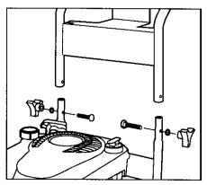
**Step 1** Attach the handle to the frame of the pressure washer. Align holes, insert bolt, add lock washer and tighten with knob.
