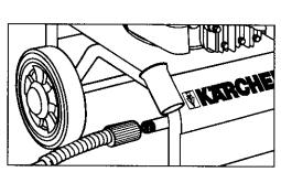
**Step 1** Connect the high pressure hose to the unit's high pressure outlet.
