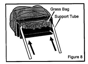
5. Push the **support tube** and bag through the front opening until only the two ends of the support tube are visible (Figure 9).
