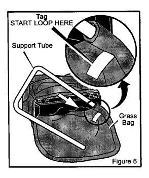
3. Slide the grass bag onto the support tube until the grass bag material is gathered onto one side of the support tube (Figure 7).
