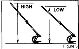
The mounting holes in the lower handle are offset (Figure 1). To change the hole offset, rotate the lower handle. This will change the angle of the handle and make the height of the handle higher or lower (Figure 3).
