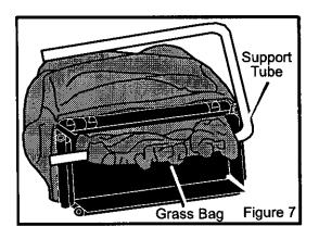
Continue to slide the grass bag onto the support tube until the grass bag material is gathered onto the top of the support tube (Figure 8).
