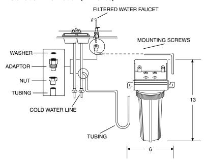
**Note:** Can be installed undercounter (as shown), in basement, or other convenient location. See installation instructions packed with product for complete details.
