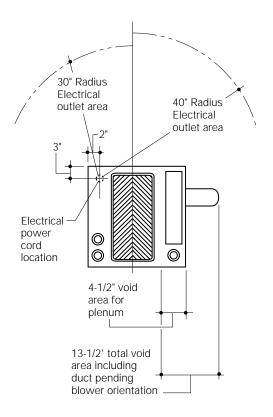
Important Information: Multiple component installations require joiner strips between components. Add 1/4" to total cutout for each downdraft vent-to-component connection; add 3/4" to total cutout for each component-to-component connection. See Monogram Component Cooktop Installation Instructions, Pub. No. 49-8834 for specific installation requirements.
