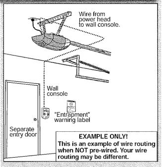
FIG.3-1 Wall Console wire routing
