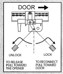
FIG. 6-3 Engage/Disengage Carriage Lock.
