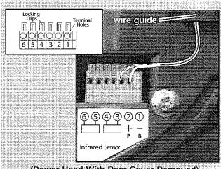
(Power Head With Rear Cover Removed) FIG. 3-3 Insert wires.
