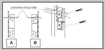
FIG. 2-8 Examples of door bracket positioning.
