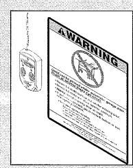
FIG. 3-5 Mounting Entrapment warning label.
