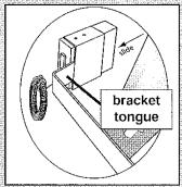
FIG. 4-3 Attach Safe-T-Beam® to brackets
