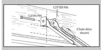
FIG. 2-5 Rail mounting to header bracket.
