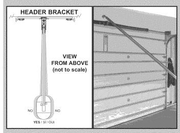
FIG. 2-4 Position assembly and align.
