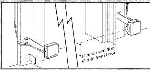
FIG. 5-4 Check Safe-T-Beam® alignment.
