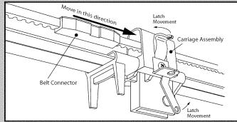
FIG. 6-2 Engage Chain/Belt Connector to Carriage.
