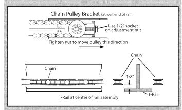
FIG. 1-6 Chain adjustment.
