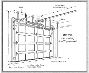
FIG. 4-6 Wire routing.
