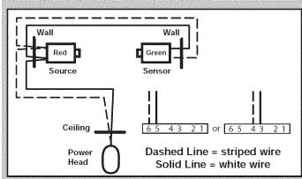
FIG. 4-5b Pre-Wired source and sensor wiring methods.
