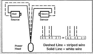
FIG. 4-5a Source and sensor wiring methods.
