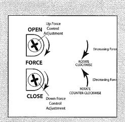
FIG. 6-5 Force Control Adjustment.
