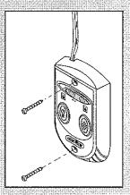
FIG. 3-4 Mounting Wall Console.
