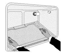
Use the finger openings along the outside edges of the oven bottom to remove the oven bottom.
