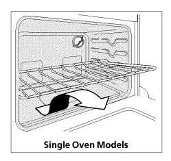
Some models have 2 flat racks. Other models have one flat rack and one offset rack. The rungs on the offset rack are slightly raised from the edges of the rack. This raised part of the rack is designed to allow easy and safe removal of foods from the lower racks of the oven and prevent hands from contacting the hot oven door. Always use the offset rack in the lower position.
