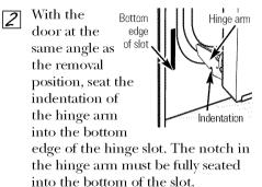
Fully open the door. If the door will not fully open, the indentation is not seated correctly in the bottom edge of the slot.
