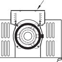
Secure the first vent component to the water heater with one self-tapping screw at the hole located above the condensate collector.
