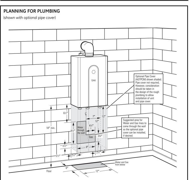
The center of the pipes can be placed anywhere within the shaded area. The center of the pipes is recommended to be protruding only within 6" of the mounting wall. Other specific installations may be different.
