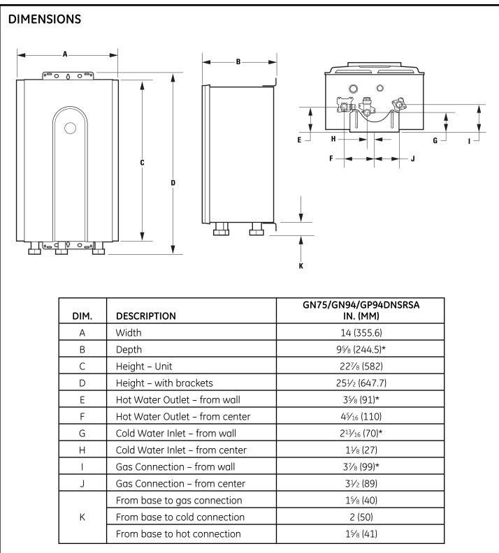
\*This is the minimum dimension from the wall. The wall bracket is adjustable to allow an additional 1.57 inches (40 mm).
