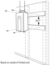
FINISHED WALLS (Drywall) Option 2: Framed wall with boards behind the drywall. Mount the unit to boards in the wall. Do not use the screws provided to mount through drywall. Screws long enough to penetrate the drywall and provide at least 1" of engagement in wood should be used. Screws should be rated to carry a tensile load of 200 lbs each. Level the unit during installation.
