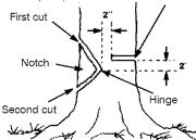
After removing the wood from the notch, make the felling cut on the opposite side of the notch. This is done by making a cut about two inches (5 cm) higher than the center of the notch. This will leave enough uncut wood between the felling cut and the notch to form a hinge. This hinge will help prevent the tree from falling in the wrong direction.
