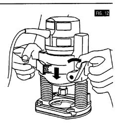
4.The desired depth of cut may now be achieved by plunging the router until the depth rod contacts the selected stop on the turret.
