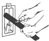
3. Place the hose clamp over the washer drain connector. Push the drain hose onto the washer connector. Use pliers to open clamp and slide clamp over drain hose. Check for good fit.
