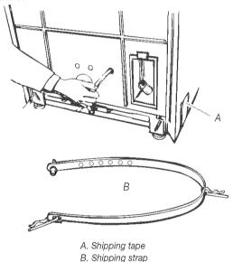
Pull firmly to remove the end of shipping strap from the back of the washer. The shipping strap plug must be completely removed from the washer for the self-leveling legs to be released.
