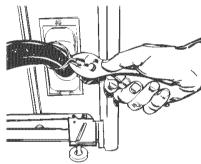
**4.** Measure and mark a point approximately 16 inches (40.6 cm) from the plug end of the shipping strap. Cut the shipping strap at this point.
