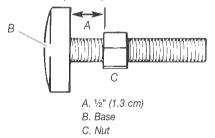
Insert legs into correct holes at each front corner of washer until nuts touch washer. Do not tighten nuts until the washer is leveled.
