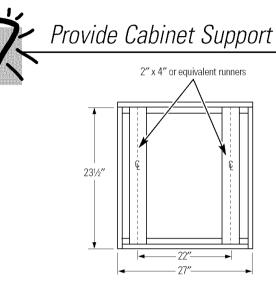
**IMPORTANT:** When installed below a single or double oven, check to be sure that any oven supports above the cutout do not obstruct the 23½" required depth of the warming drawer cutout.
