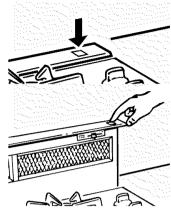
On some models, the RAISE/LOWER switch is located at the top right of the vent.
