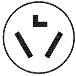
3-wire receptacle (10-30R)
