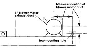
Transfer measurements and cut duct opening in cabinet floor or wall depending on your installation.
