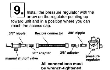
**10.** Assemble the flexible connector from the gas supply pipe to the pressure regulator in order: Manual shutoff valve, 3/8" nipple, 3/8" adapter, flexible connector, 3/8" adapter, and 3/8" nipple.
