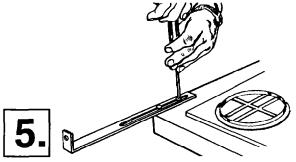
Use a Phillips screwdriver to remove the screws that attach the legs to the blower box. Place the slotted area of legs over the area where the screw openings are located. Replace the screws but Do Not tighten screws.
