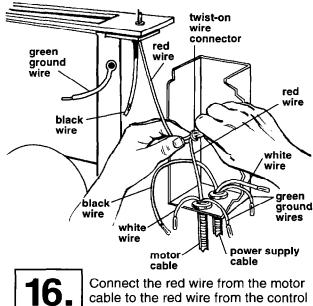
cable to the red wire from the control with a twist-on wire connector.
