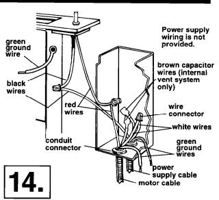
Disconnect power supply. Thread the power supply cable through the conduit connector. Tighten the screws on the conduit connector. Connect the two, white wires together with a twist-on wire connector.
