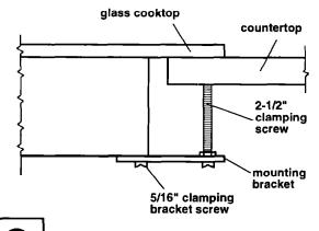
8. One cooktop in cutout: Rotate the mounting brackets away from the burner box. Do Not overtighten screws. Tighten the mounting brackets to the burner box. Insert the 2-1/2" clamping screws into the mounting brackets. Use a screwdriver to tighten the screws against the underside of the countertop. Remove the pencil outline from countertop.
