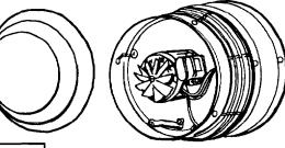
Remove the dome top. Loosen conduit connector screws. Thread the motor cable through the conduit
