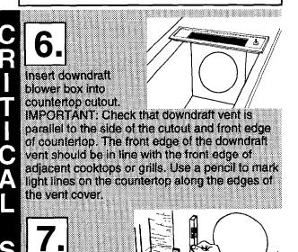
Lower legs to floor of cabinet. Place a level against the face of blower box. Adjust position of
