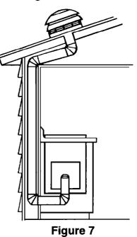
One exterior power vent motor can be used to operate two downdraft vent systems. The motor can be operated by either downdraft vent control. A T-vent Adapter Kit, (Black 4175456, White 4319251, Almond 4319252) must be used and is available from your dealer or authorized parts distributor. The maximum length of the ductwork including elbows for a T-vented system is 45 feet. The T-vent is the equivalent of 10 feet. Instructions for installing a T-vented system are included with the kit.
