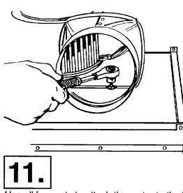
Use all four nuts to attach the motor to the blower box. Use a 10 mm or 3/8" ratchet to tighten the nut located inside the duct opening. Be sure to tighten this nut or vibration may occur, causing noise during operation.
