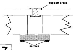
Attach support brace to side of the cooktop that will be adjacent to another appliance. Insert additional cooktop into the cutout and align with the pencil line used for first cooktop. Check that cooktop is parallel to the front edge of the countertop. Lift the entire cooktop to make adjustments so the foam sealing strip can seal properly. Repeat for additional cooktops or grills.
