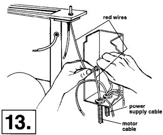
Connect the red wire from the motor to the red wire from the control with a twist-on wire connector.
