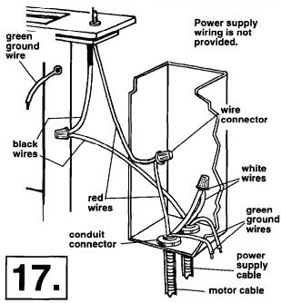
Thread the power supply cable through the conduit connector. Tighten the screws on the conduit connector.
