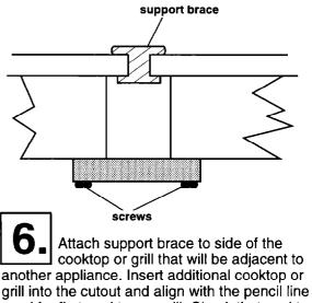
used for first cooktop or grill. Check that cooktop or grill is parallel to the front edge of the countertop. Lift the entire cooktop or grill to make adjustments so the foam sealing strip can seal properly.
