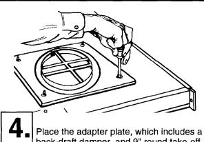
back-draft damper, and 9" round take-off on the blower box. Use all four nuts to attach the adapter to the blower box.
