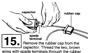
cap of the capacitor. Attach one wire to one of the inside capacitor terminals. Then attach the other brown wire to the other capacitor terminal. Replace the rubber cap over the top of the capacitor. Put the capacitor into the mounting bracket on the lower section of the wiring box.
