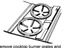
Remove cooktop burner grates and caps package from shipping box. Remove pressure regulator and hardware package from side of carton. To avoid scratching countertop, lift entire cooktop up from cutout when repositioning cooktop into countertop opening.
