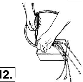
Thread wires from the motor conduit through conduit connector and through the opening of the wiring box. Tighten the conduit connector screws.
