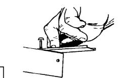
4 al Attach mounting brackets to each side of the burner box with the 5/16" screws. Do Not tighten the screws. Turn the mounting brackets so each is under the burner box. If you are installing additional appliances in the same cutout, attach one mounting bracket to the right side of each additional appliance.
