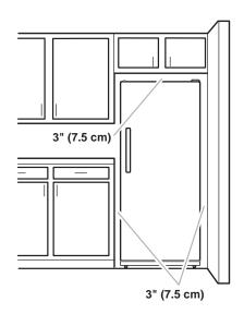
Allow at least 3 in. (7.5 cm) of air space at the top and on both sides of the convertible refrigerator/freezer and 1 in. (2.5 cm) between the back of the convertible refrigerator/freezer and the wall. If the convertible refrigerator/freezer is to be against a wall, leave extra space on the hinge side so the door can open wider.
