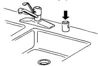
The drain air gap is usually located on top of the sink or countertop near the dishwasher. To order a drain air gap call 1-800-366-7278 and ask for Part Number 300096.
