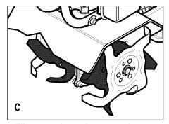
Figure 9: "A" - all four tine gangs in standard pattern; "B" - two outer gangs removed for narrow tilling; "C" - the two inner gangs have been swapped for stony tilling conditions.
