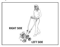
LEFT and RIGHT sides of the tiller are from the operator's position behind the handlebars (unless noted otherwise).
