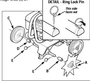
Figure 4: The Border/Edger tine (A) can be mounted on left or right sides of machine (with long bushing B). The Border/Edger wheel (C) mounts on the other side (with short bushing D).
