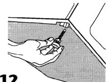
Insert legs into correct holes at each front corner of washer until nuts touch washer. **DO NOT** tighten nuts until Step 15.
