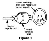
For your personal safety, this appliance must be earthed. This appliance is equipped with a power supply cord having an earthing plug.
