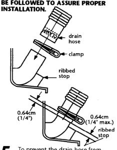
To prevent the drain hose from coming off or leaking, it must be installed per the following instructions.
