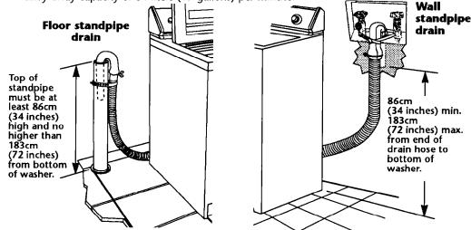
ia, use drain hose extension kit (Part No. 285/02). If drain hose must be shortened, use kit (Part No. 285442) Both kits are available from Whirlpool-authorized parts distributors.
