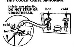
Attach bottom hose (inlet marked "H") to hot water faucet. Attach top hose (inlet marked "C") to cold water faucet. Adapters may be necessary to connect the hoses to the faucets. Tighten couplings to faucets. **DO NOT OVERTIGHTEN**; this could cause damage to couplings.
