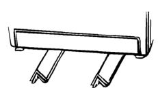
Stack two corner posts on top of each other. Tilt washer backwards and insert corner posts 7.6 cm (3 inches) from one side of washer as shown. Repeat with other corner posts on other side of washer.
