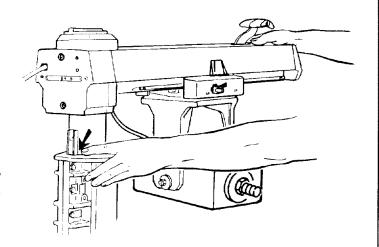
2. Loosen (2) 1/4 - 20 Gib socket cap screws on the left side at the rear of the column support slightly (1/2 turn).
