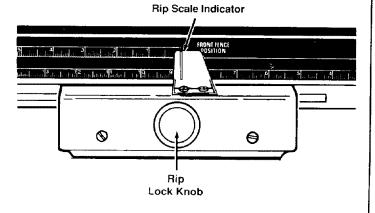
6. The blade "Out-Rip" scale indicator on left hand side of the radial arm is adjusted in essentially the same manner as blade "In-Rip" indicator, except position blade with 2 inches between fence and face of saw blade. The rip-scale indicator should be positioned to read 2 inches on upper portion of the blade "Out-Rip" scale.
