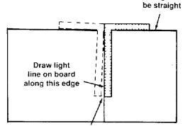
Should be no gap or overlap here when square is flipped over to dotted position.
