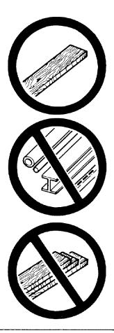
3. Rip only workpieces longer than the diameter of the blade. Do not rip workpieces that are shorter than the diameter of the blade being used.
