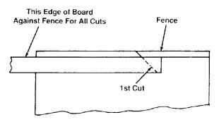
Turn Workpiece Over End For End...Keep Same Edge Against Fence When Making Successive Cuts.
