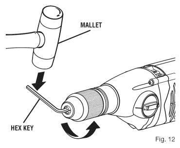
Insert the hex key into the chuck and tighten the chuck jaws securely. Tap sharply with a mallet in a counterclockwise direction. This will loosen the chuck on the spindle. It can now be unscrewed by hand.
