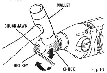
Open the chuck jaws and remove the hex key. Using a screwdriver, remove the chuck screw by turning it in a clockwise direction.
