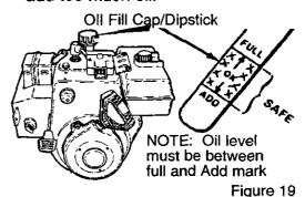
4. Tighten the fill cap/dipstick securely each time you check the oil level.
