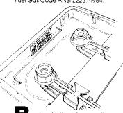
Input ratings shown on the serial/rating plate are for elevations up to 2,000 feet. For elevations above 2,000 feet, ratings should be reduced at a rate of 4% for each 1,000 feet above sea level.
