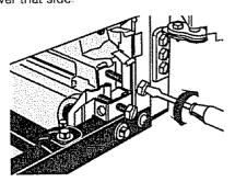
Check the door alignment after leveling the refrigerator.
