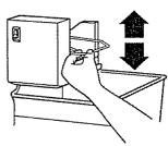
For normal ice production, set the switch on the front of the ice maker to NORMAL. In the normal ice production mode, the ice maker should produce approximately 7 to 9 batches of ice in a 24-hour period.
