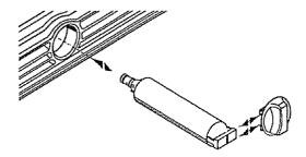
5. With cartridge cap in the vertical position, push the new filter cartridge into the base grille until it stops. Rotate the cartridge cap clockwise to a horizontal position.
