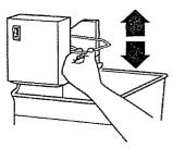
2. Flush the water system by dispensing and discarding 2 to 3 gallons (approximately 6 to 7 minutes) of water through the dispenser. This will clean the system and help clear air from the lines. Additional flushing may be required in some households.  Turn on the ice maker by opening the freezer door and lowering the wire shut-off arm as shown. Allow 24 hours to produce the first batch of ice. Discard the first three batches of ice produced.
