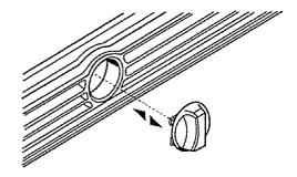
Rotate the cartridge cap to a horizontal position.
