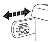
IMPORTANT: If food starts to freeze, move the control to the left (less cold). Remember to wait 24 hours between adjustments. Doing so gives the temperature of the food time to change.
