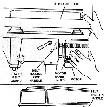
4. Loosen Belt Tension handle by turning clockwise.
