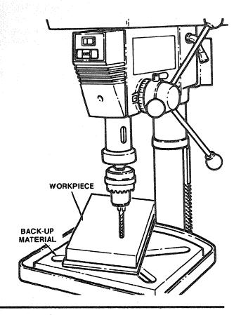
For small pieces that cannot be clamped to the table, use a drill press vise (Optional accessor). WARNING: THE VISE MUST BE CLAMPED OR BOLTED TO THE TABLE TO AVOID INJURY FROM SPINNING WORK AND VISE OR TOOL BREAKAGE.
