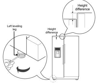
If the freezer compartment door is higher than the refrigerator compartment door, make them level by inserting flat blade screwdriver into the groove of the right leveling leg and rotating it clockwise.
