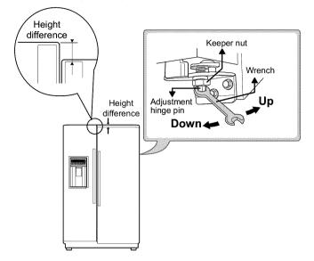
Using a 5/16" (8 mm) wrench, turn the adjustment hinge pin clockwise or counterclockwise to level the refrigerator and freezer door.
