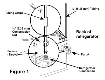
Fasten the tubing into the tubing Clamp attached to the back of the refrigerator.
