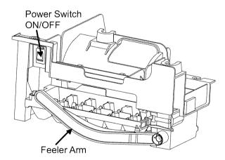
The icemaker will produce 12 cubes per cycle, approximately 140-150 cubes in a 24-hour period, depending on freezer compartment temperature, room temperature, number of door openings and other operating conditions.
