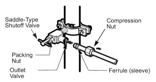
**NOTE:** Commonwealth of Massachusetts Plumbing Codes 248CMR shall be adhered to. Saddle valves are illegal and use is not permitted in Massachusetts. Consult with your licensed plumber.
