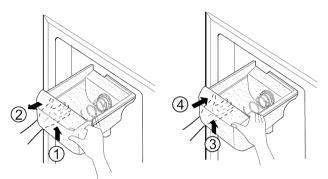
• To assemble the ice storage bin, lift it ③ while slightly pushing it in ④.
