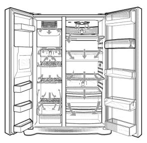
• Do not block any of these vents with food packages. If the vents are blocked, airflow will be interruped and temperature and moisture problems may occur.
