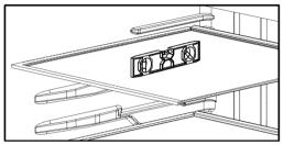
If your refrigerator is not level, insert a flat blade screwdriver into the grooves of the leveling legs (shown in picture below). Rotate legs clockwise to raise or counterclockwise to lower the front of the refrigerator.
