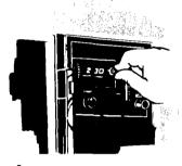
4. Set cooking times up to 10 minutes by pushing in the timer knob and turning clockwise. The oven light will go on. To set time for less than 30 seconds, turn timer past 30 seconds, then back to desired time.
