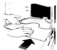
Slide the foil under the bake element.
