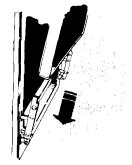
Fit the bottom corners of the door over the ends of the hinges.
