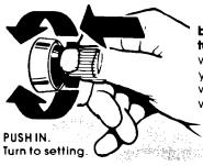
Control knobs must be pushed in before turning. Turn either way until the setting you want shows in the window. Set them anywhere from HI to OFF.
