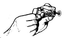
First make sure lower oven and surface unit control knobs are set on OFF. All knobs pull straight off. Surface unit knobs have a collar and spring.
