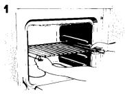
Lift rack at front and pull out.
