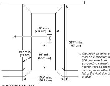
1. Grounded electrical outlet must be a minimum of 3" surrounding cabinets or nearby walls as shown. It can be placed either to the left or the right side of the
