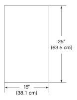
Panel should be 1/2" (13 mm) min. thickness
