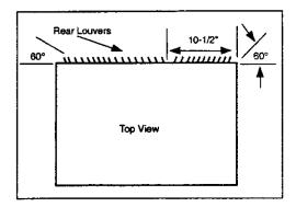
1. Redirect the louvers at the back of the wall sleeve as shown in the illustration. The use of pliers is recommended.
