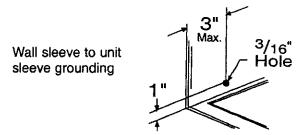
4. Prepare the wall sleeve for installation of the new unit per the following Brand instructions.
