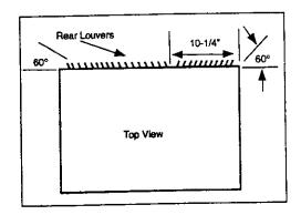
Redirect the louvers at the back of the wall sleeve as shown in the illustration. The use of pliers is recommended.
