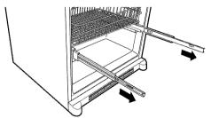
**B** Locate the slots on the inside of the rail assemblies near the back.
