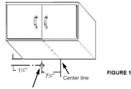
1½" dia. clearance hole in wall for recommended power supply location
