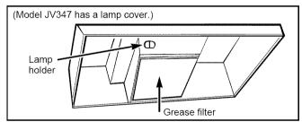
Your hood is equipped with a metal grease filter. When the fan is operated, air is drawn through the filter and discharged to the outside.
