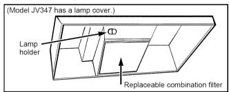
Your hood is equipped with a replaceable combination filter. When the fan is operated, air is drawn through the filter and discharged into the room through the hood.
