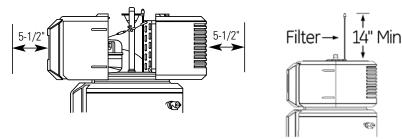
A 14" minimum clearance is required to remove the filter for cleaning. The hot and cold water plumbing and electrical connections must not interfere with the removal of the filter.
