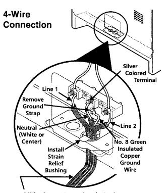
4-Wire Copper Power Supply Cord. To Fused Disconnect Box or Approved Wiring Device for Copper Supply Cord.
