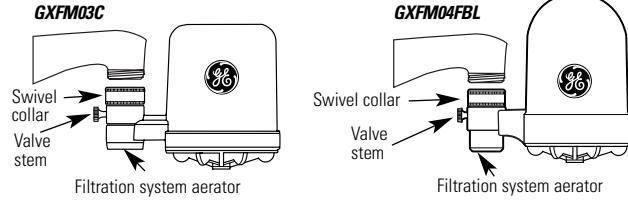
**4** Slowly turn on the cold water (about half open) and check for leaks. Tighten as necessary. Enter filter installation date on change filter reminder and place on calendar at 3 months from install date.
