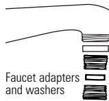
■ **Internal threads** – Use trial and error to select the proper adapter and washer combination. Screw adapter and gasket onto faucet. Be careful not to cross thread the adapter; tighten manually.
