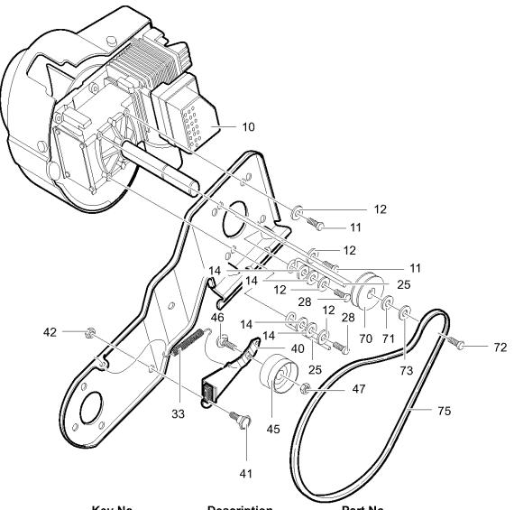
Key No. Description Part No. 10 (SEE ENGINE MANUAL) **ENGINE** 180077 11 SCREW, 5/16-18 X.75 12 WASHER 120638 WASHER, FLAT 71071 14 25 GUIDE, BELT 313440 28 **SCREW** 710312 33 SPRING, IDLER BRAKE 165x146 40 ASSY, IDLER ARM 1501013 41 **BOLT** 333594 42 NUT, 5/16-18 71391 45 PULLEY, IDLER 48924 46 **BOLT, CARRIAGE** 45892 47 NUT 590 70 PULLEY, ENGINE 338849 71 WASHER 25840 72 SCREW, 5/16-24X.75 181595 73 WASHER 120638 **BELT** 760928 75
