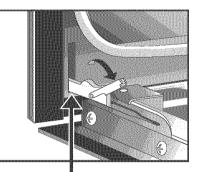
Lock engaged for door removal
