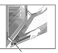
**HINGE SLOT - Door removed** from the appliance
