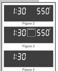
The (model) or (m) pad controls the Broil feature. When broiling, heat radiates downward from the oven broiler for even coverage. The Broil feature is preset to start broiling at 550°F however, the Broil feature temperature may be set between 400°F and 550°F.
