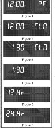
The 🐨 or 🝈 and 🖙 or 🕟 pads control the Continuous Bake or 12 Hour Energy Saving features. The oven control has a factory preset built-in 12 Hour Energy Saving feature that will shut off the oven if the oven control is left on for more than 11 hours and 59 minutes.
