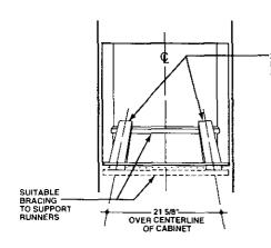
If the cabinet does not have a solid bottom, then two braces or runners must be installed to support the weight of the oven. For single ovens the runners and braces must support 150 pounds.
