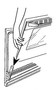
The oven door is heavy. You may need help lifting the door high enough to slide it down onto the hinges. Do not lift the door by the handle.
