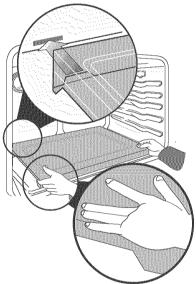
Grasp the oven bottom by the front corner on each side to raise and lower the oven bottom.
