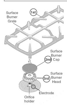
**To Remove and Replace the Surface Burner Caps and Burner Heads -** Remove in the following order: (1st) surface Burner Grates, (2nd) Burner Caps and (3rd) Burner Heads. Replace in the following order: Burner Heads, Burner Caps and Burner Grates.
